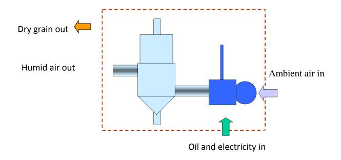
In grain drying the moisture in the grain moves to the air, which is blown through the grains
